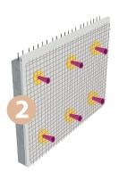
The strut cones are placed trough the distribution washer. The frame is set up.
