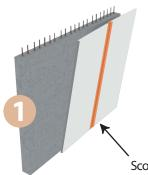
The panels are positioned against the first concrete wall. Threaded rods go trough the cardboard.
