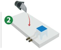
Concrete is poured around the REZABOITE G.
