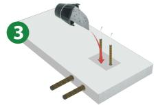
Opening of the REZABOITE P. Passing of the PE, connection to the network and filling the box.
