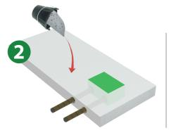
Pouring concrete around the Rezaboite P. The ducts are protected.
