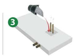
Opening of the REZABOITE G. Passing of the PE, connection to the network and filling of the box.
