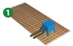
The legs of the REZABOITE G are cut to fit the thickness of the slab. The REZABOITE G is placed on the formwork base and tied to the mesh (in pre-slab: the legs are folded and spiked with a metal strip).
