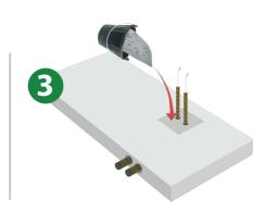
Opening of the REZABOITE G. Passing of the PE, connection to the network and filling of the box.
