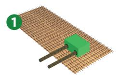
Installation of Rezaboite P directly on the welded wire mesh (hold by ligature). Incorporate the sheaths / sleeves.
