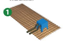
The legs of the REZABOITE G are cut to fit the thickness of the slab. The REZABOITE G is placed on the formwork base and tied to the mesh (in pre-slab: the legs are folded and spiked with a metal strip).
