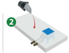
Concrete is poured around the REZABOITE G. The ducts are protected.
